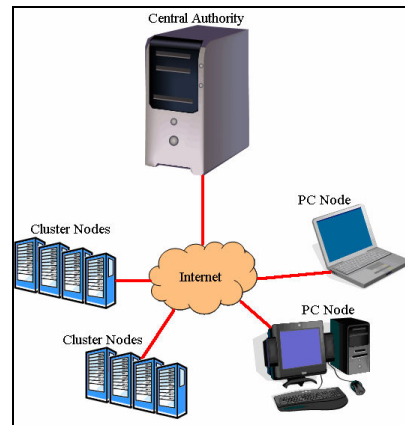
Figure 1 - Grid Architecture Example
